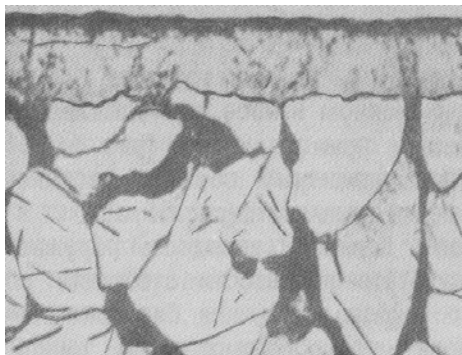
Fig. 9. The microstructure of nitrocarbonized EN C15 steel at 570 °C for 2 hours.
